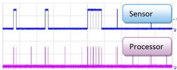
Based on an oscilloscope reading, the top image shows how a processor programmed by us specifically alternates between sleep mode and active data processing. When developing a system, it is essential to monitor the residual charge. Accordingly, we were also able to achieve a battery lifespan of 10 years for the three AA cells of type Li/FeS in the motion detector shown below.
